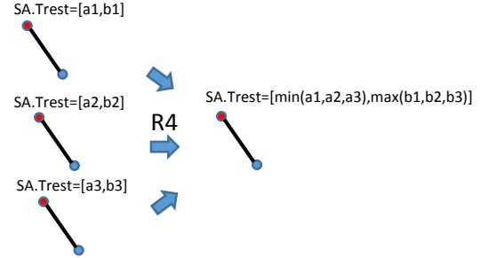
Figure 12: Rule 4: Merging parameter ranges
